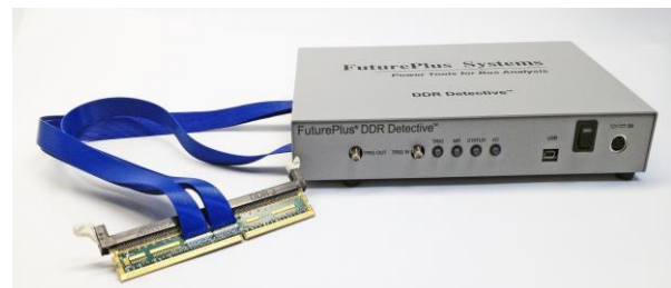
Figure 3: The repurposed DDR Protocol Analyzer with its DIMM interposer
