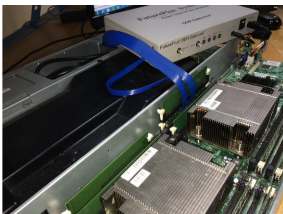
Figure 3: Open Compute Server being tested for Row Hammer failures
