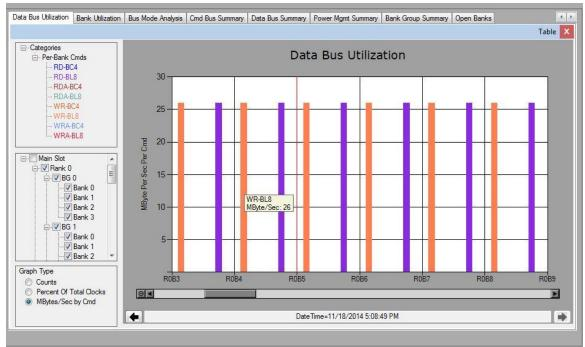
Figure 5: DDR4 Data Bus Bandwidth by Bank
