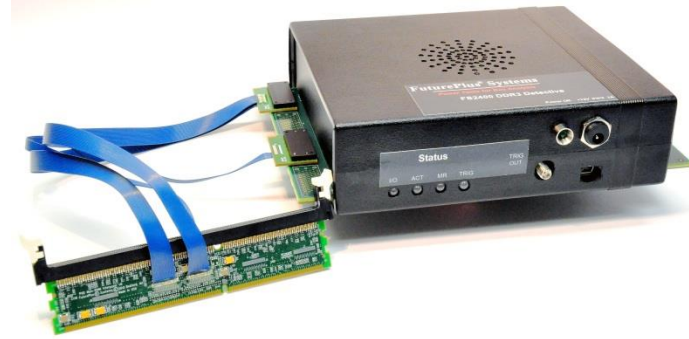
Figure 4: The DDR3 Detective® with DIMM interposer from FuturePlus Systems
